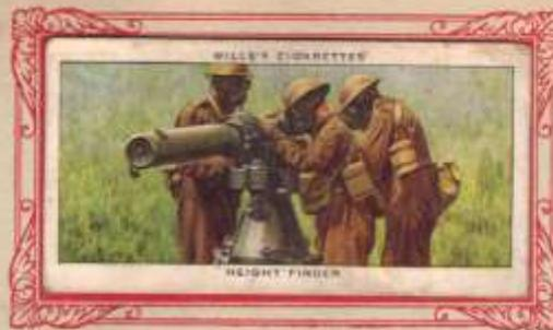
THE HEIGHT-FINDER is an essential part of the equipment of the Anti-Aircraft Gun Section, for on the skill of the men working it the whole success of the shooting rests. Our picture shows an instrument with a base length of 9 ft. being operated by its crew of 3, who are wearing gas masks. This is a modern instrument and is being issued in considerable quantities to Territorial Anti-Aircraft Units for Home Defence. (No. 49)
